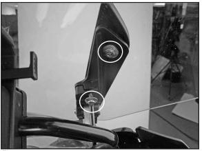
7. Secure windshield with stock screws. **Tighten Firmly**. Repeat procedure on left side. **(T25 Torx) Figure 8**
